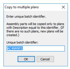
Unique batch identifier is automatically generated. You can use this one or rename the batch as you need.
