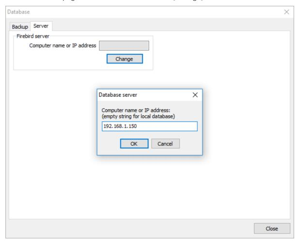
Fill in computer name or IP address where Firebird SQL server is installed and click the [OK] button.
