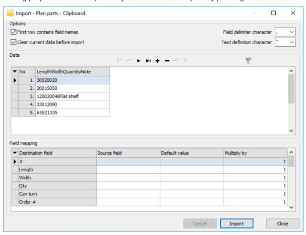
Here you have to setup options in order to format source data from the clipboard to the form suitable for the fields mapping. In our case we have activated option First row contains field names and we have set Field delimiter character to TAB value.
