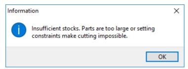
Solution is to split these parts. Select all parts (CtrI+A) and choose the menu item "Edit > Split part". Enter desired length (in our case 1,000,000) and press "Split" button. Parts are split into following fragments.
