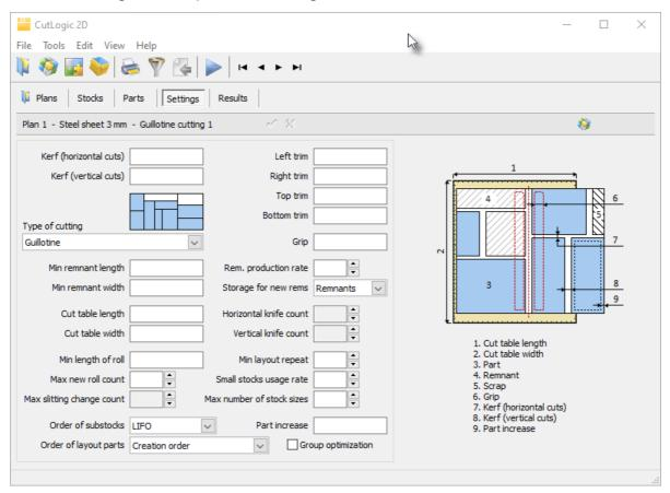
Settings tab enables you to define cutting settings for given plan.
