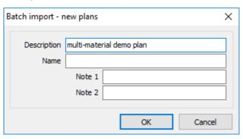
Confirm [OK] and program automatically creates multi-material plans from imported parts.
