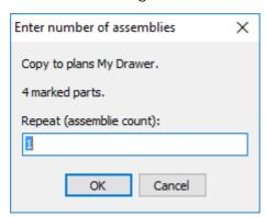
Here you can change repetition of copied assemblies. The original quantity of parts will be multiplied by entered value. Confirm the dialog to create plans.
