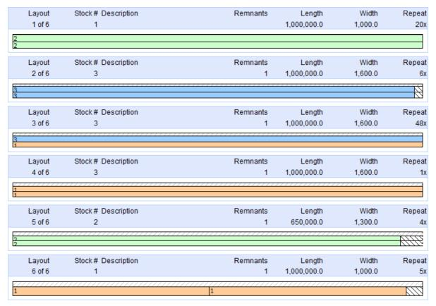
After optimization of cutting plan which includes split parts, UI and "Cutting layouts" report show how to cut material to get part fragments. After the part fragments are cut, you need to put them together and join them to get final parts.
