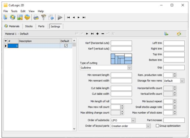
Settings tab enables you to define list of pre-defined plan settings for given material. See more in chapter  $\underline{\text{Entering Settings for the Plan}}^{(86)}$ .
