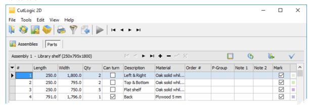
Parts tab enables you to define parts for given assembly. Parts in assemblies represent bill of materials or customer orders. This is new point of view on how to work with parts. It can be very useful in cases when you prepare cutting plan with many assemblies or orders. This feature brings time saving and simplifies preparation of the new cutting plan.
