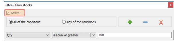
The filter will display only the records which fulfill defined conditions. Activation of filter is signalized by the red labeled information in toolbar.
