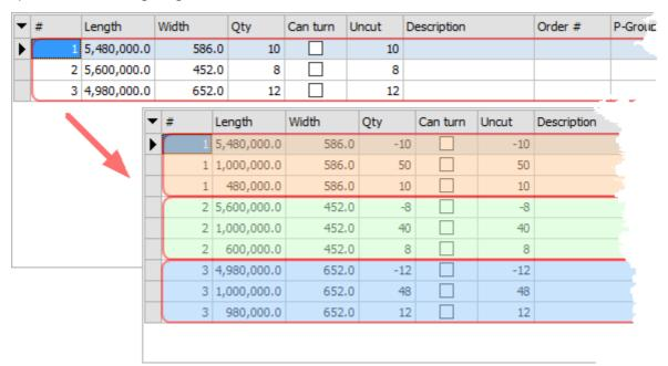
As you can see, all part fragments have the same Part # as their original part and are recognized via this number. Now it is possible to run optimization. Following diagram demonstrates optimized plan.
