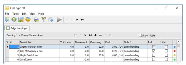
Edgebands tab enables you to define edgebands or it can be used for defining of post-processing of parts (e.g. grinding). Once you define edgebands you can assign them to edges of plan parts. See also <u>Defining edge banding</u> (82).
