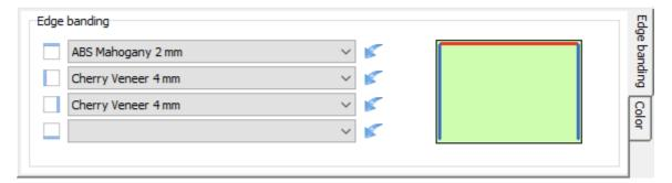
Here you can set part edge banding from predefined <u>Edgebands</u> Each of part sides can have different edgeband. Colored lines along part sides indicate defined edgebands.
